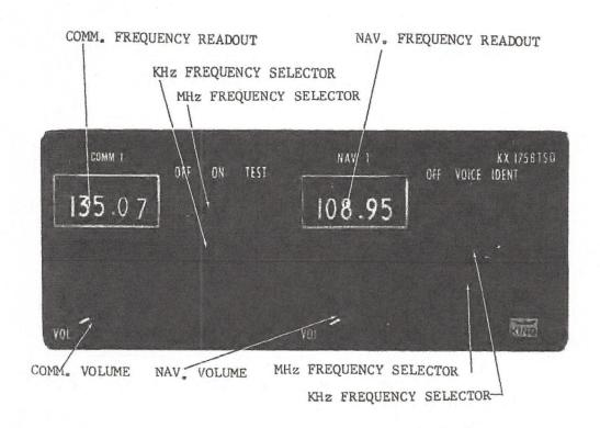
FIGURE 3-1 KX 170B/175B CONTROL FUNCTIONS
